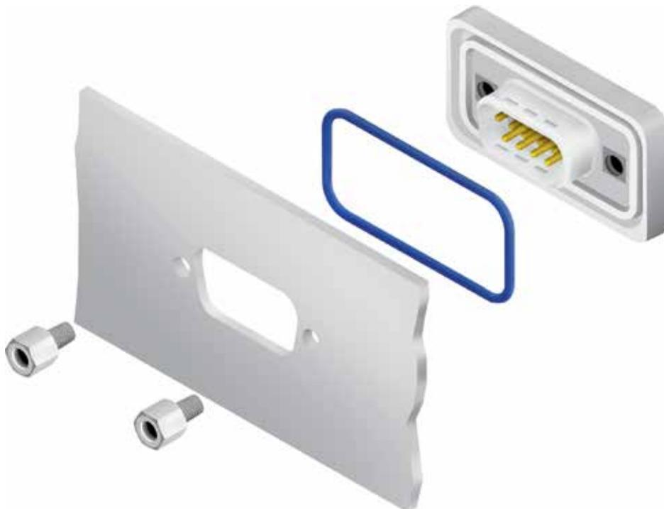
The hex bolts illustrated here (4-40 UNC or M3 threads) are included in the delivery complement of every connector with a sealing frame. The length of this spacer has been selected to accommodate a panel thickness of .063"/1.6 mm such that it does not extend beyond the plug-in height. Furthermore, the hex bolts outside threads are shorter than standard hex bolts. Material: stainless steel.
