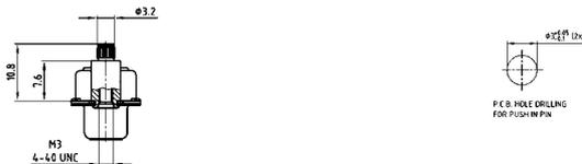
Mounting style: 4-40 UNC rear press-fit spacer
