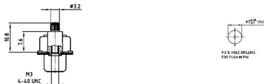
Mounting style: Rear press-fit spacer
